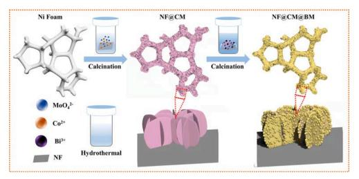
Fig. 1. Schematic illustration of the designed process of NF@CM@BM heterojunction membrane.
