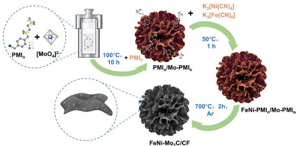
Fig. 1. Schematic of the synthesis of the FeNi-Mo 2 C/CF.
