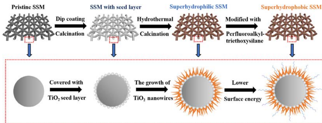
Scheme 1. Schematic illustration of formation process of superwetting mesh and cross section of the single wire.
